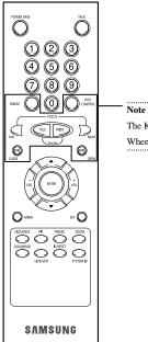
The Keys inside this line are not related with System functions. When these keys are pushed, only beep Sound are generated.
